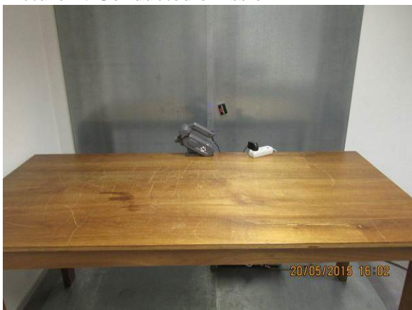
Picture 3: Conducted emission test setup
