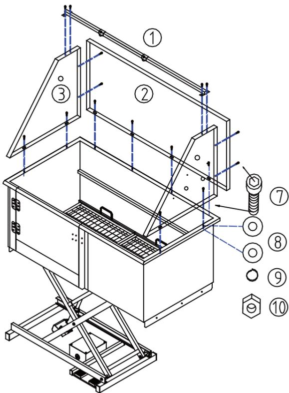
1. Bolt the bottom of the Back splash (2) to the Tub basin (4). Use an Inner hexagon screw (7), two Φ16mm Washer (8), a Spring washer (9) and a Nut (10) in every pre-drilled hole.
